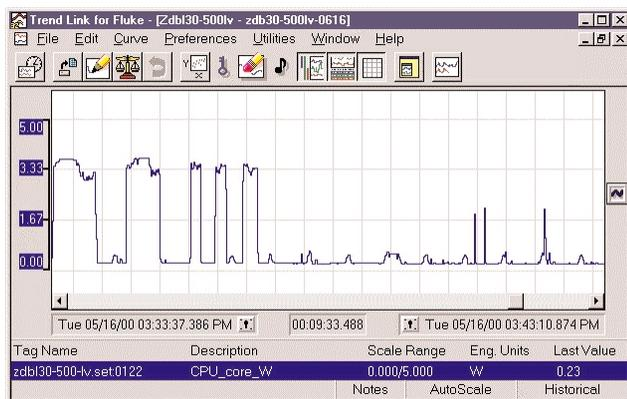
**Figure 3.** This power-consumption trace shows a 500/600MHz mobile Pentium III processor running the ZD Media BatteryMark 3.0 program, which keeps the CPU idle most of the time. That allows Intel's QuickStart power manager to reduce average power consumption well below 3W.
