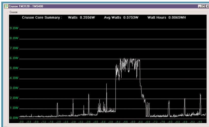
**Figure 2.** Transmeta's instrumented test system continuously plots power consumption while other software is running. This trace plots the playback of a DVD movie, with regularly spaced spikes marking the decompression and display of each video frame. The large but brief power surge was caused by launching another Windows application.
