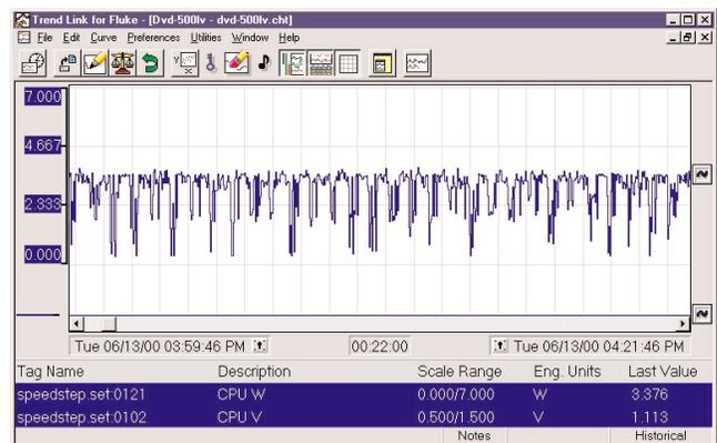
**Figure 4.** This trace shows a 500/600MHz mobile Pentium III processor playing a DVD movie in battery-optimized (500MHz) mode. Compared with the similar trace from Transmeta in Figure 2, the Intel processor appears to be consuming at least twice as much power—even without a north bridge, which would add about 4W.
